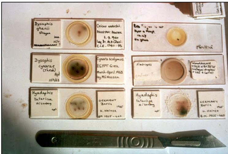
Fig. 2 Deteriorating aphid slides showing blackening and crystallization of Berlese gum choral mountant and the removal of the sealant ring with scalpel.
