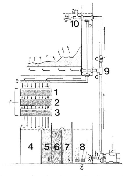
Fig. 5 The ten stages in filtration (see text) a. 'Venturi' device; b. one inch diameter over flow pipe with coarse filter' c/d/ adjustable valve and T-piece on 3/4 inch pipe balancing reverse flow between 'venturi' and under-gravel return; e. spray bar to spread water flow; f. filter trays stacked two inches apart; g. airstones to aid re-oxygenation; h. non-return valve to prevent siphoning if pump fails; i. Stuart Turner pump.
