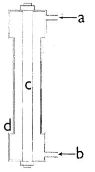
Fig. 9 Protein Skimmer. a. water from the aquarium enters the cylinder; b. diffuser; c. outlet back into the aquarium; d. protein froth; e. removable top.
