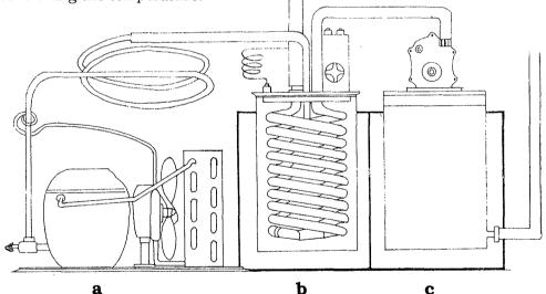
Fig. 10 Cooling system. a. compressor; b. heat exchanger; c. Eheim Power Filter.
