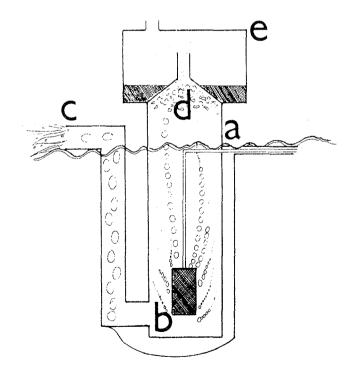
Fig. 8 Protein Skimmer. a. water from the aquarium enters the cylinder; b. diffuser; c. outlet back into the aquarium; d. protein froth; e. removable top.
