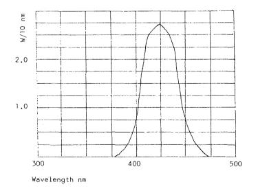
Fig. 4 Spectral analysis of actinic blue lamps.
