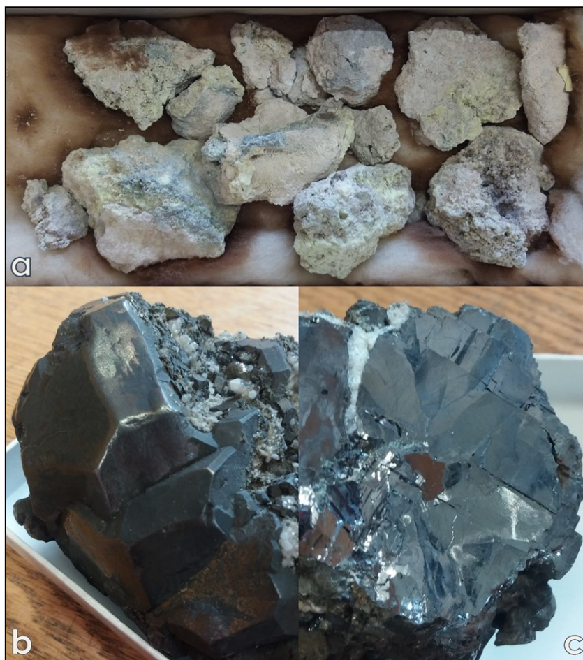
Figure 6. A. Sulfur specimen OUMHN.MIN.08345 is in multiple parts and displays noticeable cracks and crumbs. Efflorescence and a dark soot-like coating is also visible upon close examination.
